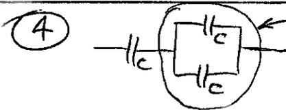
Parallel:  $C_{EQ} = C_1 + C_2 \Rightarrow C + C = 2C$
