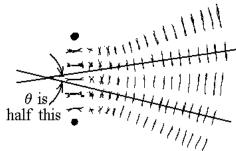
Notice the standing wave along the line between the two sources formed by the identical waves traveling in opposite directions. This is the easiest place to measure the wavelength. Each flickering bright spot is an antinode; mark as many of them as you can clearly see. Measure across them and divide to get  $\lambda$ . Also measure d, the distance between the two sources. Measure d on the screen, not at the balls themselves, to be consistent with your other measurements.
