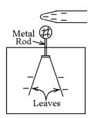
A. Charging by friction, and charging by contact. Transferring electrons by rubbing is called charging by friction. You will use this method to charge an insulating rod. Charging an object by touching it to another charged object is called charging by contact. Once you have the rod charged, you will charge the electroscope by touching it. Follow the answer sheet for details of what to do.
