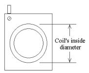
2. Wrap a piece of insulated wire around the solenoid ten times and connect it to a voltage sensor plugged into channel A of the computer interface. Connect the solenoid to Output 1 of the interface.
