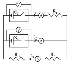
Set two of the meters to read DC volts and the other three to read DC milliamperes. Starting with their knobs all the way down (counterclockwise), turn on the power supplies then adjust them as closely as possible to the  $\mathcal{E}_1$  and  $\mathcal{E}_2$  you chose. Record the currents. A current whose direction is opposite that shown in the picture should be recorded as negative.
