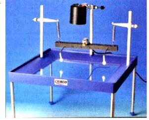
Before adding water, place the tank on an 18" by 24" sheet of paper with the extra few inches extending beyond the side opposite the vibrating bar.
