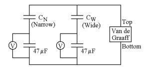
Notice that both  $C_N$  and  $C_W$  will have essentially the same voltage across them, as you assumed under "theory." Both have one plate connected to the top of the Van de Graaff, and, with only a fraction of a volt across the 47  $\mu$ F capacitors, both have the other plate pretty much at the potential of the bottom of the Van de Graaff.
