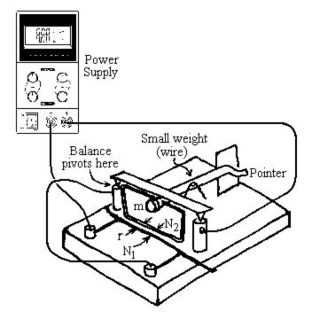
measure left to left, then right to right, then average. (Trying to measure r between these wiggly bunches of wires is the largest source of error in this experiment.) After this be careful not to move where the pivot points rest on their supports or you could change r.
